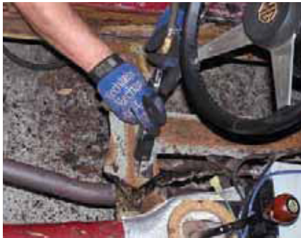
7. Using an air-powered body saw, we cut out the old pans.
