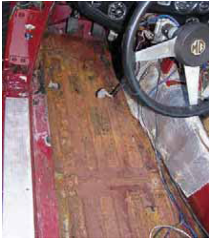
6. We began by raising the car as high and level as possible before securing it on jackstands. From underneath, we then drilled holes at the edges of obstructions. We used these holes as a guide when cutting out the old pans from above.
