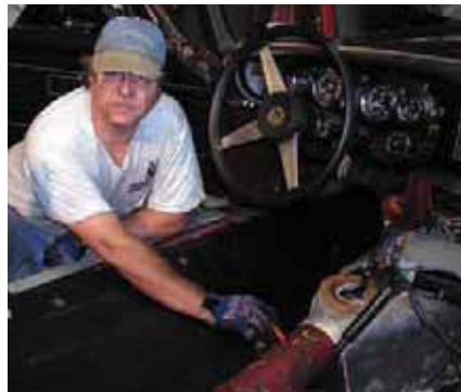
13. After several fit-and-trim procedures, we marked the edges of the body sheetmetal and braces on the pan from underneath. Using these marks, we drilled 3/16" holes about every 1.25 inches for spot welds.
