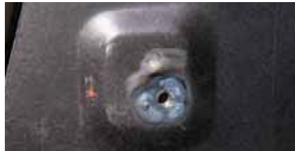
10. Use the seat rails to locate the seat nuts perfectly. If you don't get this right, you'll have to slot the seat-rail holes.
